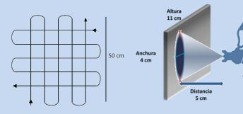
In the case of using "TransTech"-type air-forced spraying guns, it is recommended to apply **two layers** of the product, being **perpendicular among them** (see the figure) to perfectly cover all the surface.
